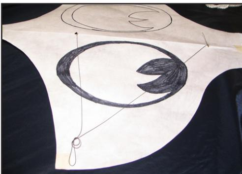
The “Bridle Point”, where your flying line attaches to the bridle, is found by stretching the bridle out to a wingtip, and making a small loop there.
